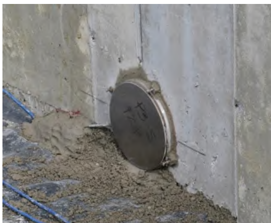
Figure 42. Photo. Lateral earth pressure cell behind the GRS abutment backwall.
